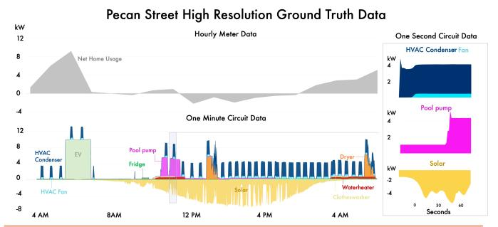
In 2025, we began capturing snapshots of voltage and current waveform data for a portion of our connected homes, which allows for detailed analysis of electrical loads, identification of specific device signatures, and detection of anomalies in electrical circuits.
