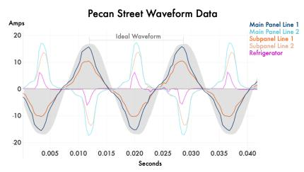
Circuits measured in millisecond reveal the shape of their waveforms
